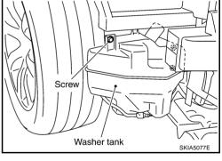
Remove washer tube, and remove washer tank from the vehicle.
