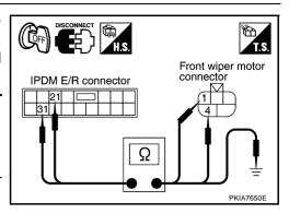
3. Check continuity between IPDM E/R harness connector terminal and Ground.
